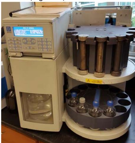
**Figure 2: Dionex ASE 300 Accelerated Solvent Extraction System**
