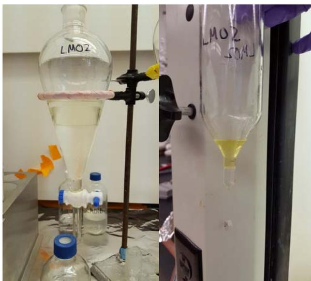
**Figure 3: (Left) Sample Present in Separatory Funnel (Right) Sample after TurboVap Treatment**
