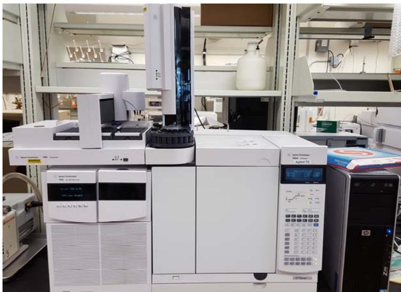
**Figure 6: Agilent 7890B GC System Equipped with 7693 Series Automatic Liquid Sampler Coupled to a 7000C Triple Quadrupole MS System.**
